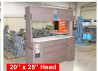
FIPI Hydraulic Press Traveling Head, 25 Ton Model F 63M-HS 64" x 25" Work Space
