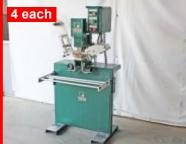
Trekk Model HT-300 Vertical Heat Transfer Press Roll to roll auto label feeder
