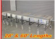
**Accordion Conveyor** Best Flex Motorized Conveyor 28" Wide Rollers, 110 volt \$995.00/\$1,850.00
