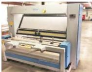
72" Inspection Machine Set up w/ edge guide, forward/ reverse, speed control, inspection light, & surface rewinder
