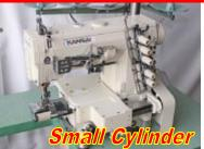
K.S. Model NM-1103CL Cyl Cover Stitch, Set up w/ Ndl Pos, Thread Trimmer, FL
