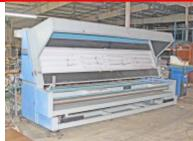
156" Inspection Machine Set up w/ electronic edge guide, forward/reverse, speed control, surface rewind, & yardage counter
