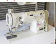
**Brother Model ZE-856A** Fully Automatic Single Needle 12 Needle, 1/4" Ga, Cyl Chain Zig Zag, Programmable Pattern
