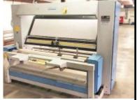
72" Inspection Machine Set up w/ edge guide, forward/ reverse, speed control, inspection light, & surface rewinder
